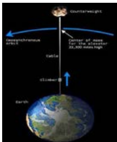
Figure 1. Scheme of the parts of the Space elevator
