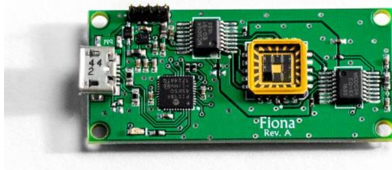
**Fig. 1.** Ocean Insight PCR Fluorescence Sensor
