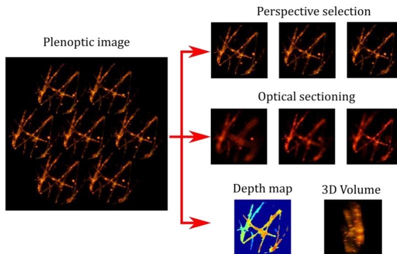
Figure 2: Plenoptic image of cotton fibers captured with the DOIT 3D Micro 1 using fluorescent illumination and different types of optical processing from that plenoptic image. From the plenoptic image, the point of view of interest can be selected, as well as a specific focused section in depth; or it can be calculated a depth map (in the figure red es close and blue far)
