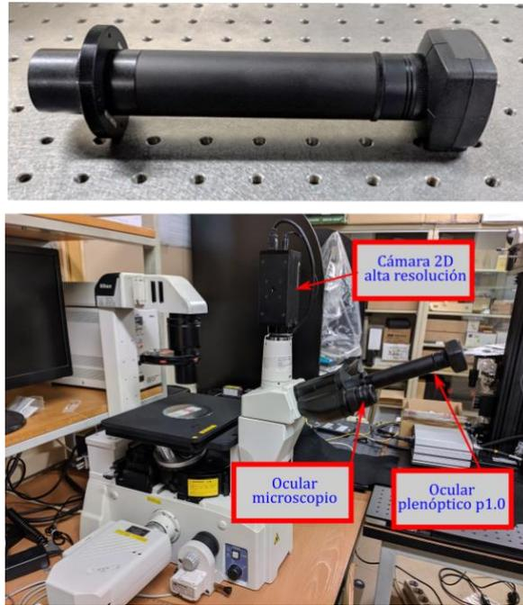
Figure 1: Pictures of the DOIT 3D Micro lab prototype (top) and the prototype coupled in the eyepiece port of a microscope (down).
