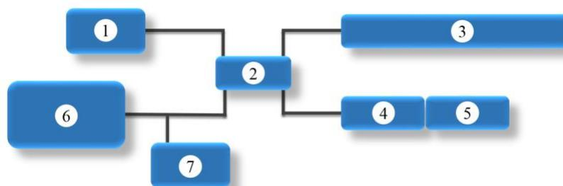
Fig. 3. Experimental layout for interferometer: 1. Supercontinuum Source SCT1000. 2. Fiber wideband Coupler 50/50. 3. Free Space Length-Tunable Arm. 4. Reference Standard Fiber. 5. Photonic Device to Characterize. 6. Optical Spectrum Analyzer. 7. Fast Oscilloscope
