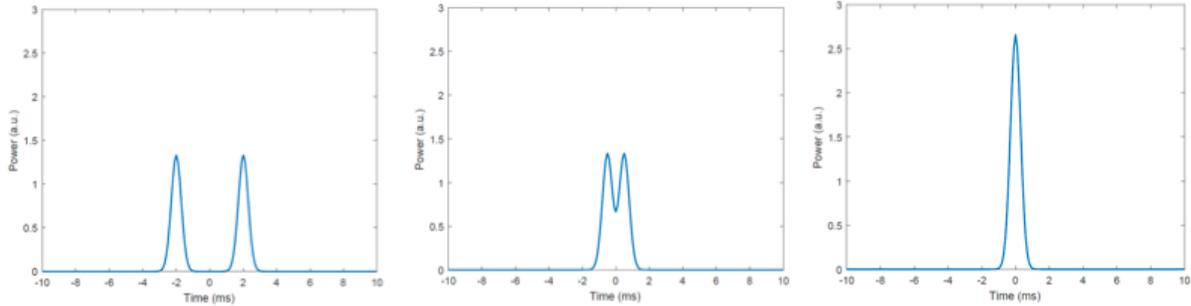
Fig. 4. In the images, from left to right, a diagram of the pulse overlapping process. Each pulse refers to a different arm of the interferometer and they gather together when you tune the length of the free space arm.
