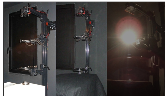
Fig. 10. Several steps of the irradiance calibration of the Brewer#201.
