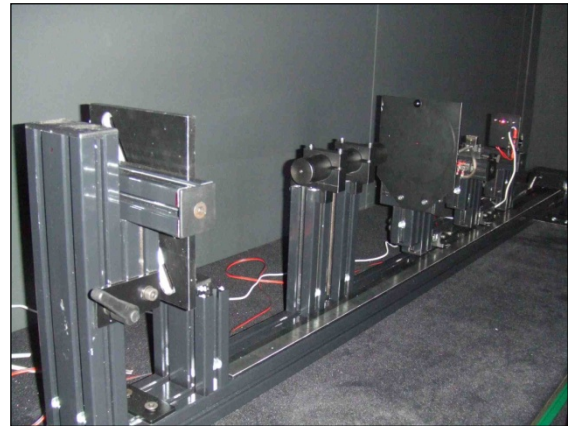
Fig. 1. Horizontal absolute irradiance calibration set-up.
