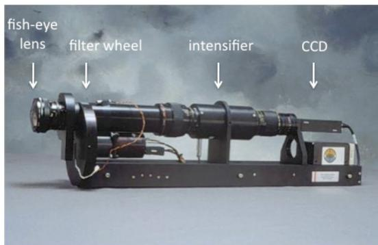
Fig. 2: Main components of an intensified CCD (ICCD) camera, manufactured by Keo Consultant.
