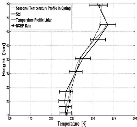
Fig. 3: Mean temperature profile computed from 40 lidar measurements in spring (black solid line) with error bars corresponding to one sigma standard deviation. Grey solid line: lidar temperature profile obtained on October 17, 2005. NCEP temperature profile above Río Gallegos on October 17, 2005 (black square).
