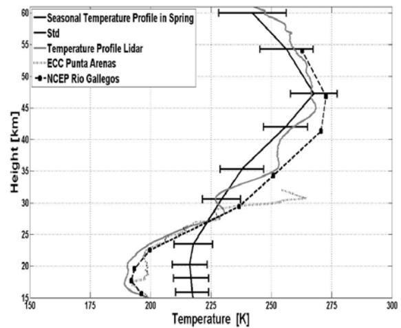
Fig. 5: Mean temperature profile computed from 40 lidar measurements in spring (black solid line) with error bars corresponding to one sigma standard deviation. Grey solid line: lidar temperature profile obtained on October 9, 2005. NCEP temperature profile above Río Gallegos on October 9, 2005 (black square) and temperature profile from ozonesonde launched in Punta Arenas-Chile (dotted grey line) are also shown.
