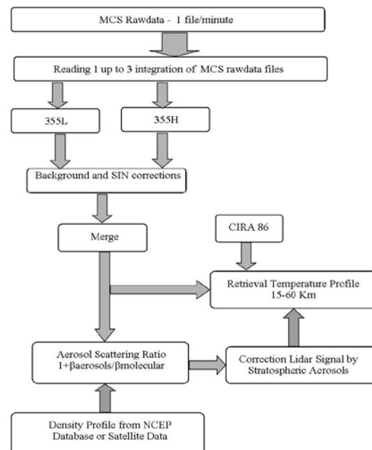
Fig. 1: Flow chart of signal processing. Different corrections are implemented to eliminate uncertainties. Temperature profile below 30 km is corrected using the ASR.
