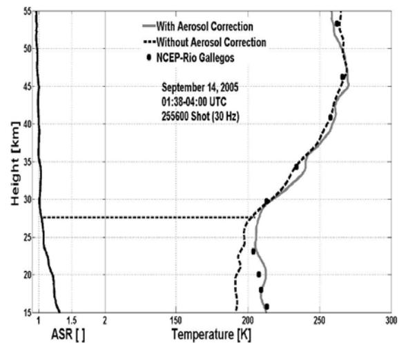
Fig. 2: (Right) Temperature profile on September 14, 2005 corrected for aerosols (grey line) compared to NCEP (black square) data above Río Gallegos. The dotted line shows temperature profile affected by aerosols. The aerosol scattering ratio profile is displayed on the left. The horizontal line separates the region of aerosol influence on lidar temperature profiles.
