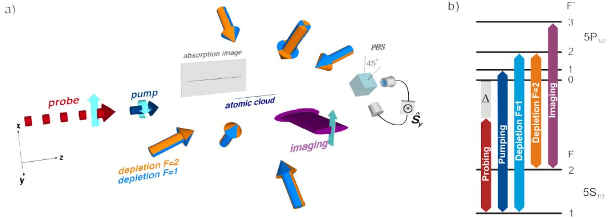
Fig. 3: a) Atomic ensemble with probing, pumping, and imaging light fields. The polarimeter measures in the 45°-basis, i.e., the Stokes component  $S_y$ ; b) Atomic transitions for probing, preparation, and imaging light fields.
