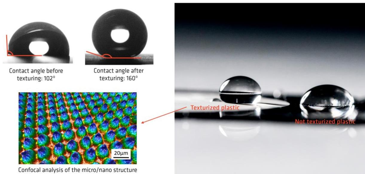
Fig. 2. Analysis of water drop over texturized and not texturized plastic (microstructure applied on mold) and confocal microscope analysis of the micro/nano structure
