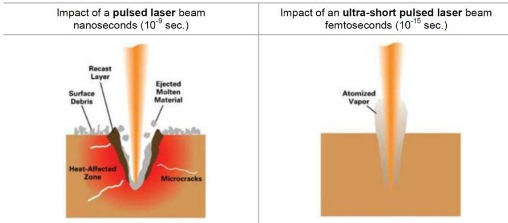
Fig. 1. Comparison of the impact of nanosecond laser vs femtosecond laser
