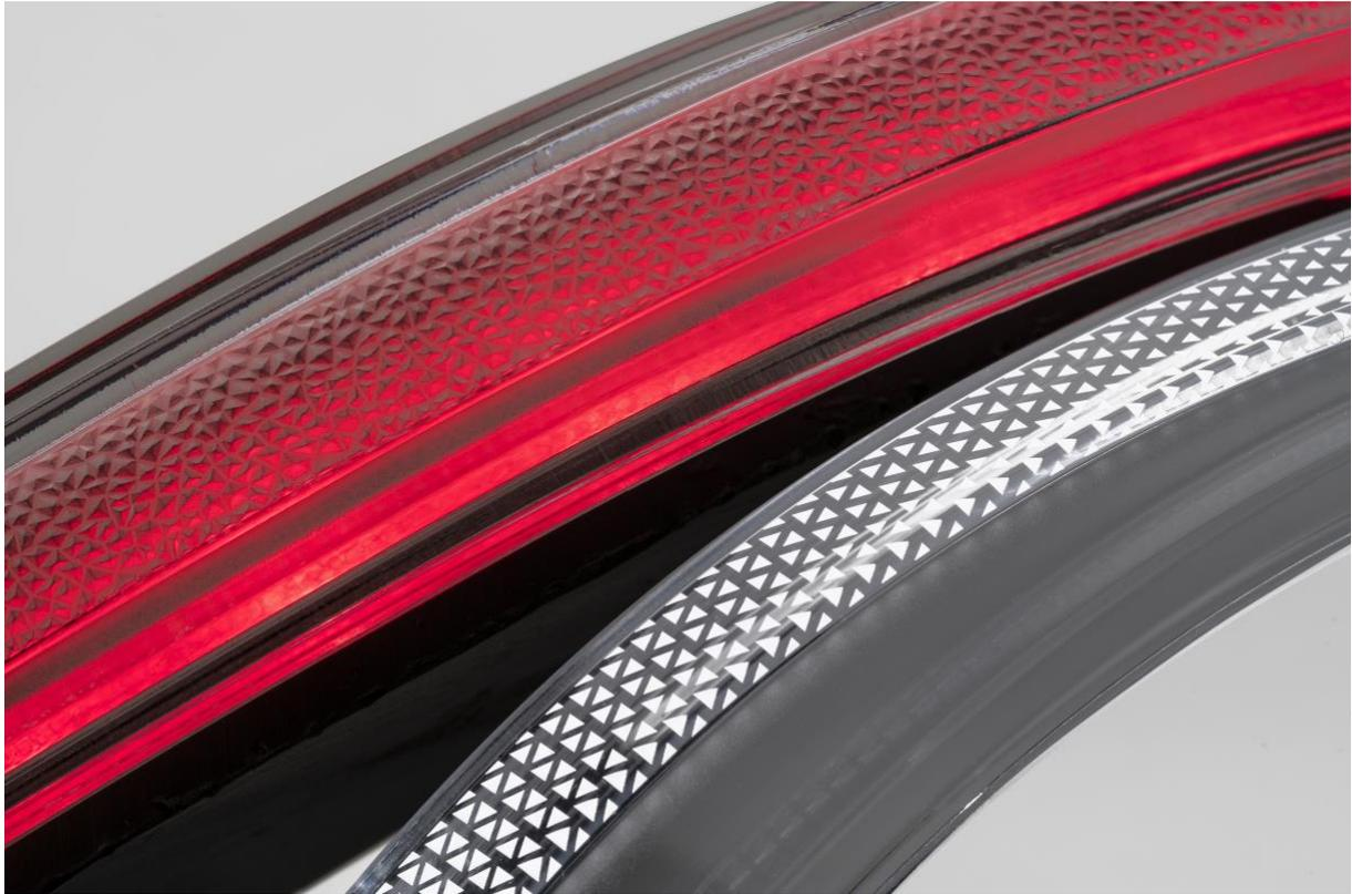
Fig. 4. Micro milling and decorative light diffusion texture over PMMA prototypes for automotive industry
