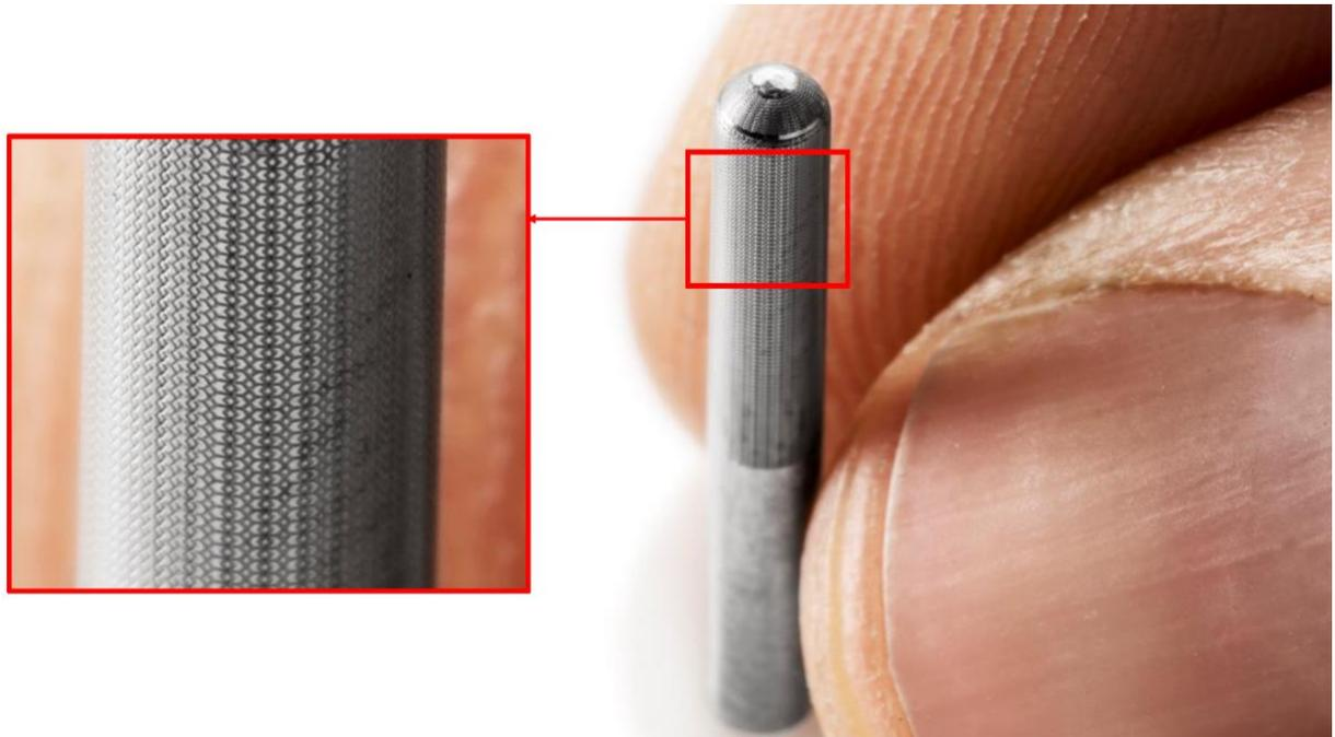
Fig. 3. Micro milling over cylindrical part for medical purposes
