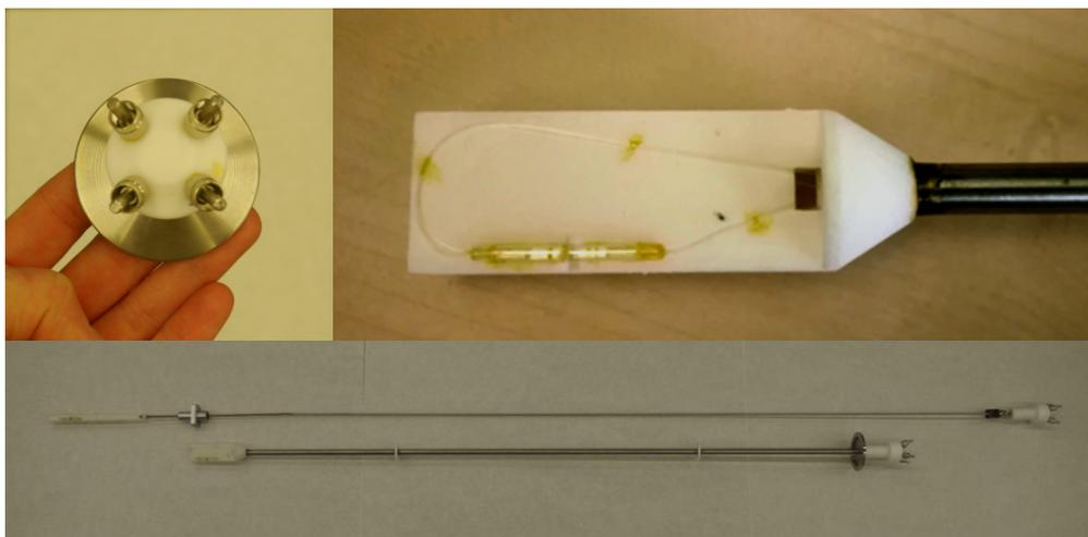
Fig. 1: upper- left corner: space sealer with 4 SMA connector. Upper-right corner: Sample holder. Bottom: two different U-specs adapted to different cryostats.
