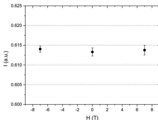
Fig. 4: Stability of the transmission data ( $\lambda = 550 \text{ nm}$ ,  $T = 70 \text{ K}$ .) under magnetic fields: relative error ( $< 0.2 \%$ ).
