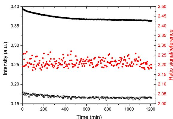
Fig. 2: Time-signal stability (ratio signal/reference in red; transmission and background signals in black: full and empty circles, respectively)
