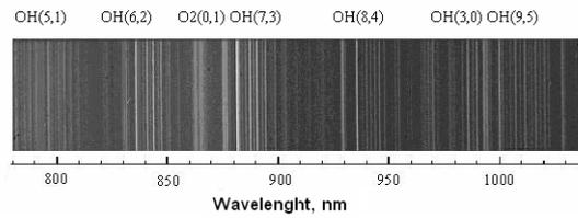
Fig. 1. The emission spectrum of the nightglow in the near infrared region. The emission bands of OH and O<sub>2</sub> molecules are indicated on the top.
