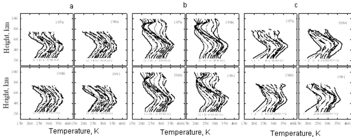
Fig. 1: Vertical distributions of the average monthly temperatures in the middle atmosphere at (a) low, (b) middle, and (c) high latitudes for the years of solar activity minimums (1976,  $F_{10.7}=73$ , and 1986,  $F_{10.7}=75$ ) and maximums (1980,  $F_{10.7}=198$ , and 1991,  $F_{10.7}=208$ ). The temperature profiles for each month are shifted to the right relative to the previous profile by 10 K. The first profile on the left corresponds to January.
