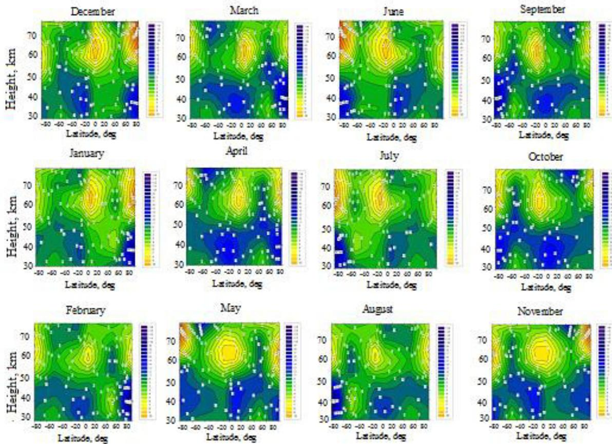
Fig. 3. The altitude distribution of the temperature response of an atmosphere on solar activity in the latitudinal range from 80 S up to 80 N for all months of year.
