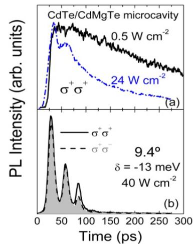
Fig. 5. Polarization-resolved emission in a CdTe microcavity at 9.4° and different power densities.
